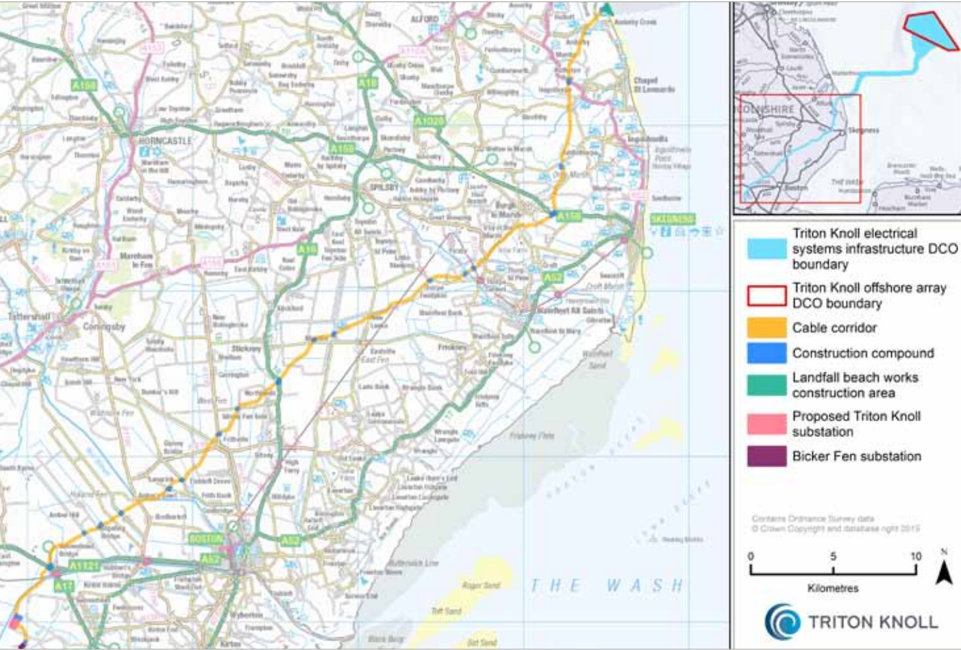
Caption: Maps shows the electrical system without the intermediate electrical compound.
